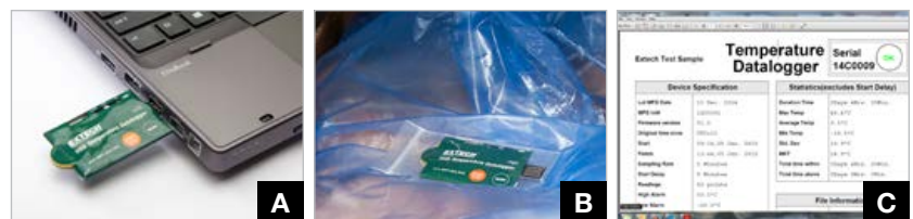
A. Plug into a PC to adjust the settings (requires Adobe® Reader® software) B. Put the Datalogger back inside plastic bag and seal the opening, then place in an area where temperature is to be monitored and press START for the unit to start recording C. When datalogging duration is completed, plug back into a PC where it will automatically generate a PDF report.
